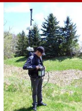
GEM Overhauser Magnetometer system. It can be configured with additional survey sensors for simultaneous gradiometer readings as well as VLF. System configurations can also include walking mode and gps.
