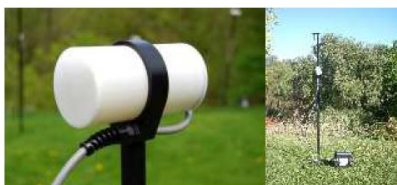
GEM-GSM-19 Overhauser Magnetometer Small and light weight. Rugged plastic housing protects the internal components during operation and transport.
